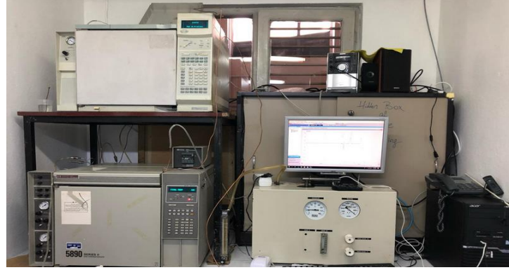
Figure 1. The experimental set up for spontaneous combustion liability determination.
